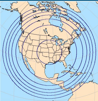
MPAS 60-3 km mesh, 58 levels, 43 km top cell spacing (c.i. 8 km, 4 km inner contour)
